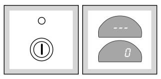
If the programme selector dial is on the RESET **O** position, three flashing dashes will be displayed. If the programme selector dial is positioned on a wash programme, a flashing zero will be displayed.
